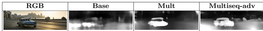
Fig. 7: Depth maps extracted from the predictions of the three models for a specific RGB image of KITTI Dataset. Note that the colors in the predictions of the models have been inverted for a better visualization i.e. closer pixels are whiter while further pixels are darker. (KEY: Base model has been trained only with images taken from Cam 5; Mult model’s training involves images from Cam 2, Cam 3 and Cam 4; Multiseq-adv model is our proposal, as it has been trained using images from Cam 2, Cam 3 and Cam 4 and it includes adversarial training for camera generalization).
